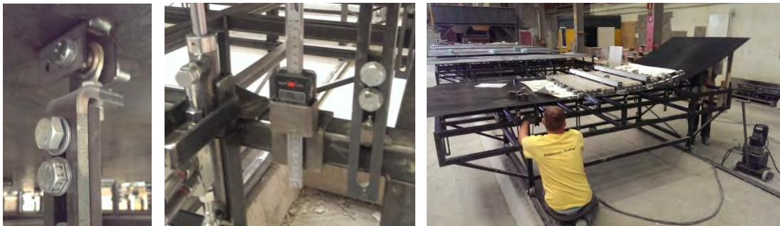
Figure 17, 18, 19: Adjustable pin construction flexible mould
