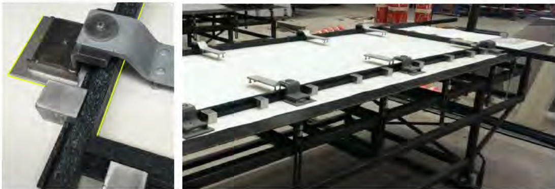
Figure 15, 16: Laser projection for the placement of edges and brackets
